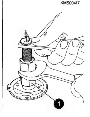
Checking commutator end shield
